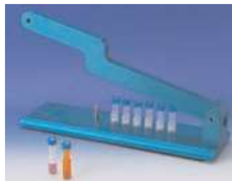
The Mini-UniPrep filter on the left is shown with fluid in the chamber. On the right, the filter plunger is shown compressed with the sample ready for analysis.
