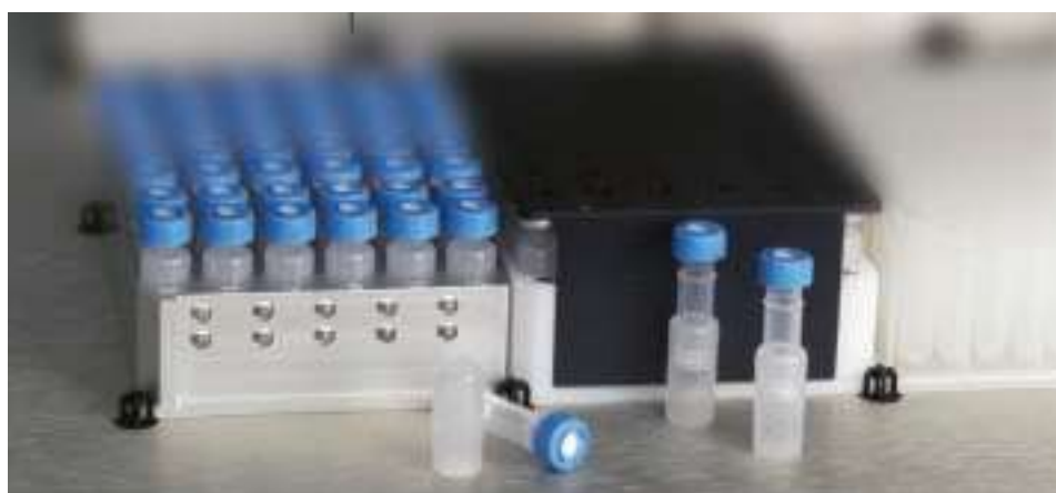
The Mini-UniPrep filter on the left is shown with fluid in the chamber. On the right, the filter plunger is shown compressed with the sample ready for analysis.
